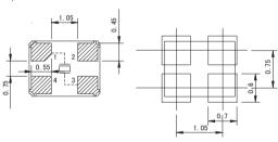
Note) #2, #4 is connected with a cover (Please connect with a GND or a power supply)
